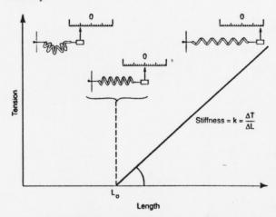
The slope of the line shown in the figure, the incremental force  $(\Delta F)$  corresponding to a unit change in length  $(\Delta L)$ , represents the spring constant k, also known as the stiffness.
