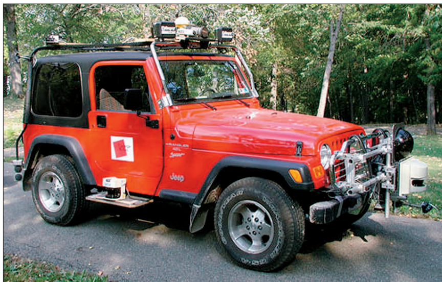
Figure 4. A Navlab vehicle developed at Carnegie Mellon University can autonomously operate at high speeds for an extended period of time. (figure courtesy of CMU and Red Whittaker)
